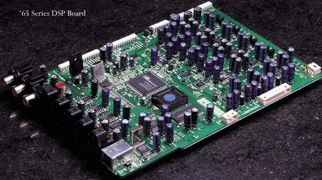
P-965, R-965 "Analog Devices" Chips Note: AD-1896 Digital Remastering Chip & AD-1852 24/192 Audio DAC's
