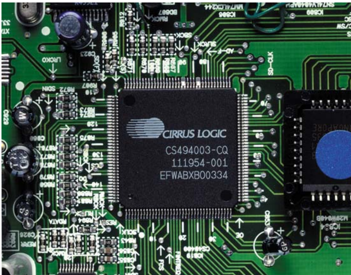
Close-up, 32-Bit CS-49400 DSP Processor Chip. This chip is found in the P-965, R-965 & R-865
